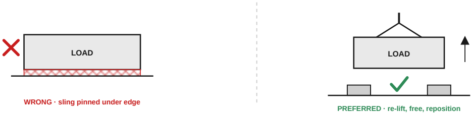
Fig. 3 — A trapped sling is a re-lift, not a reach
