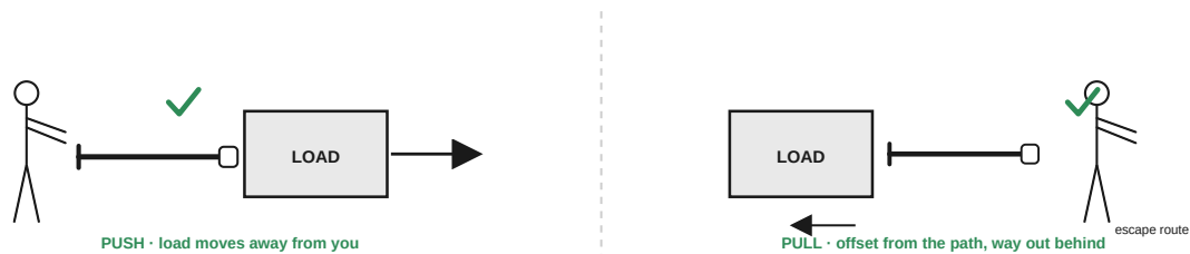
Fig. 4 — Push with the load moving away; pull from the side
