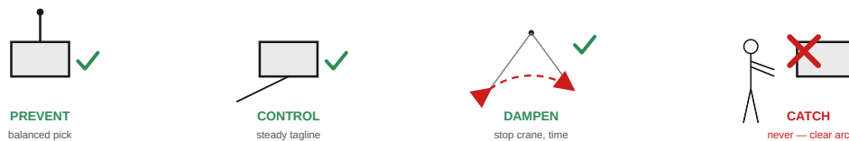
Fig. 3 — Prevent, control, dampen — never catch
