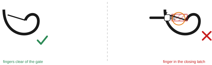
Fig. 3 — Keep fingers out of the latch as it closes
