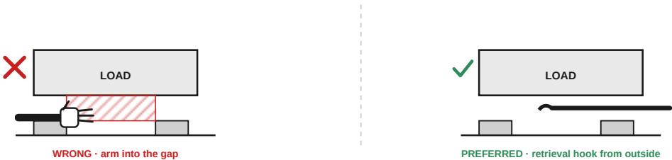
Fig. 5 — For a free but awkward sling, use a tool not an arm
