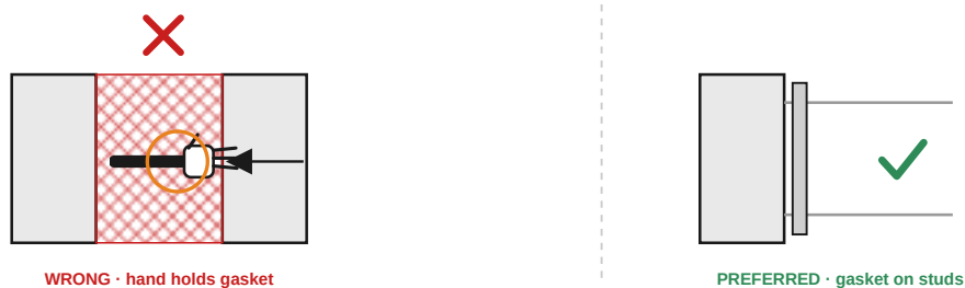
Caption: Fit gaskets and shims with the gap wide and on guide studs — never hold them by hand as the gap closes.
