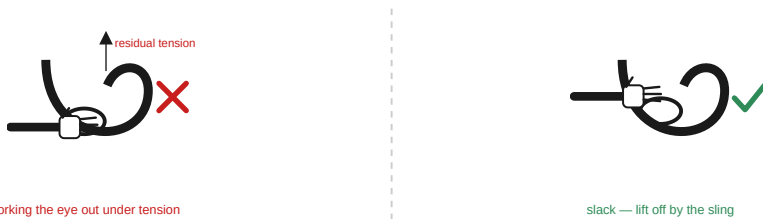
Fig. 5 — Take the sling off only when it is fully slack
